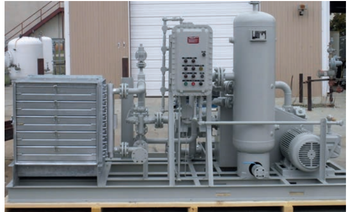
Corken HG601AA fuel gas compressor package.
