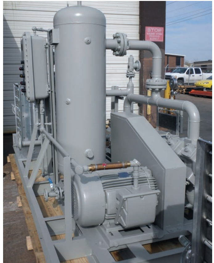
Tank serves as both pulsation dampener and inlet liquid trap (discharge tank by others)
